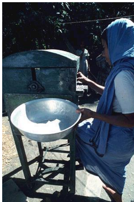
Figure 2: Grating coconut with a treadle powered machine in Bangladesh. Photo credit Practical Action / Neil Cooper
